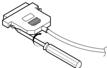
1-8-3 Attach the other end of the cable to the computer.
