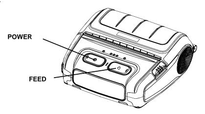
While the printer is turned off, turn on the printer while pressing the feed button. The printer setting values will then be printed.
