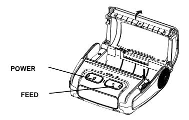
Turn on the printer while holding down the feed button like self test mode. Then close the cover to enter hexa dump mode. The below message is printed.
